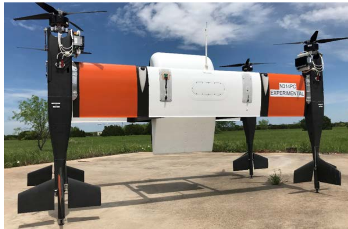
Figure 2.2.2-1: The Bell Textron (Fort Worth, Texas, U.S.A.) APT70 unmanned aircraft.
